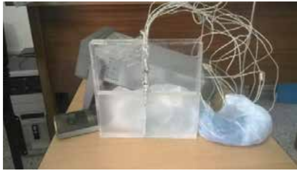
Figure 2. PCM wall filled with Paraffin-27.
